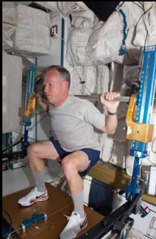
Steve Lindsey, STS-133, 2011 aRED, Advanced Resistive Exercise Device Max load (2675 N),
